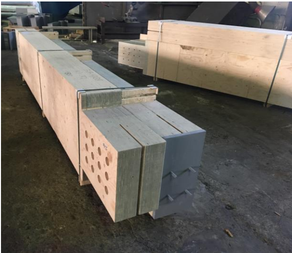
Figure 43: Left: Bolted connection for LVL G columns in production (Wood city project, Finland); Right: Screwed connection for LVL G trusses in production (Ydalir project, Norway)
